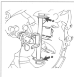
1.1 Clutch release pivot shaft - BE3 transmission
